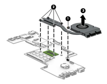
NOTE: The thermal material must be thoroughly cleaned from the surfaces of the fan/heat sink assembly and the system board each time the fan/heat sink assembly is removed. Thermal material is used on the processor (1) and the fan/heat sink assembly section (2) that services it.
