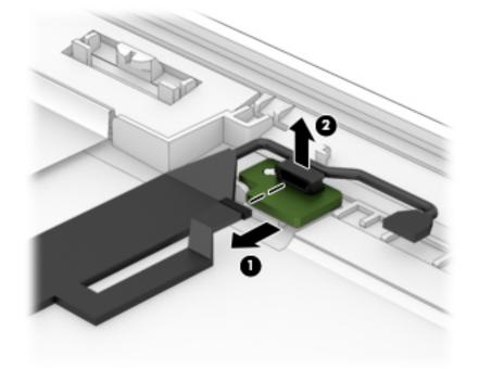
f. Remove the display LED board.
