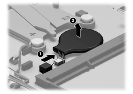
Reverse this procedure to install the RTC battery. When installing the RTC battery, make sure the "+" sign faces up.
