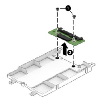
Reverse this procedure to reassemble and install the solid-state drive.
