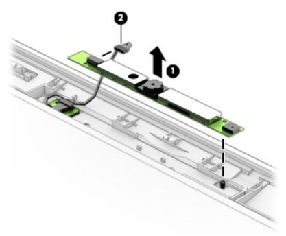
d. Remove the webcam/microphone module.
