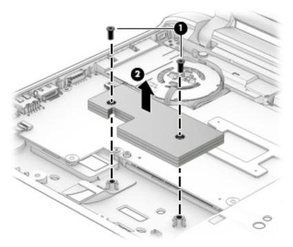
Reverse this procedure to install the counterweight.
