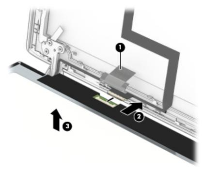
**14.** If it is necessary to replace the display LED board:
