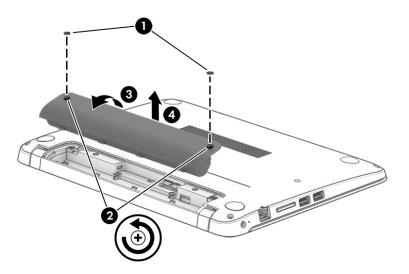
Reverse this procedure to install the battery.
